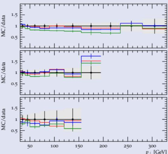
Transverse momentum of the first, second and third jet (from top to bottom) in  $W^\pm + \geq 1, 2, 3$  jet production as measured by ATLAS compared to predictions from the corresponding fixed order and MC@NLO simulations.
